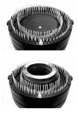
Figure 25: Upper: Unloaded spider. Lower: Loaded spider showing the bending strain on the inner roll and in plane strain on the outer roll. The contour of inner pins bents and the outer pins remain still.
