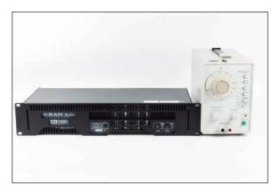
Verify the compression driver (8  $\Omega$ ) by applying a 3.5 V amplitude signal and make a frequency sweep starting at 200 Hz up to 20 kHz.
