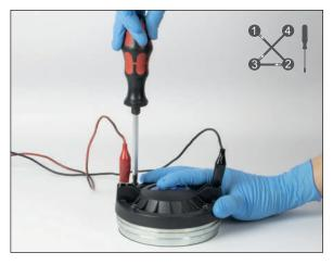
Place the diaphragm and the screws. Apply a 200 Hz signal of 3.5 V amplitud. Move the diapghragm carefully to that position where no distortion is percibed and screw progressively in the order indicated in the diagram.
