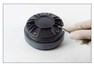
Unscrew the screws and remove the cover and the diaphragm you want to replace. It is highly recommended to clean the air gap using adhesive tape.
